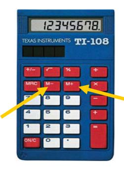
The [M+], [M-], and [MRC] calculator keys. The [M+] key is used to add a number to the number stored in the calculator's memory; the [M-] key is used to subtract a number from the number in memory. The [MRC] key, pressed once, displays the number currently stored in memory; when the key is pressed twice, the calculator's memory is cleared.
